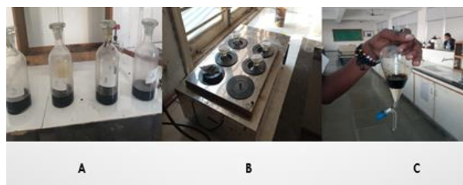
temperature 60(±)2°C), B - Temperature optimization by heating samples up to 90(±)2°C, C - Separation of water and oil phase
