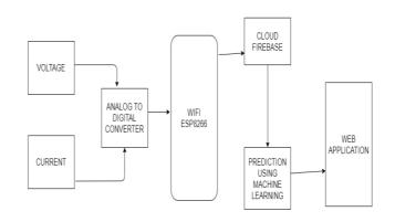
A smart metre is an electronic device that keeps track of data like electric energy usage, voltage levels, current, and power factor. Smart metres provide data to consumers for better understanding of usage patterns, as well as to energy suppliers for system monitoring and customer invoicing. Smart metres generally capture energy in close time and send out reports at regular intervals throughout the day.
