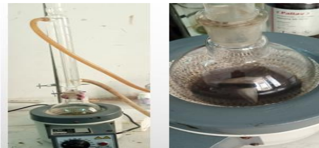
Figure 4 : Determination of Asphaltene content
