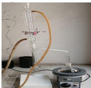
Figure 1 : Dean and Stark Method for determination of water content.
