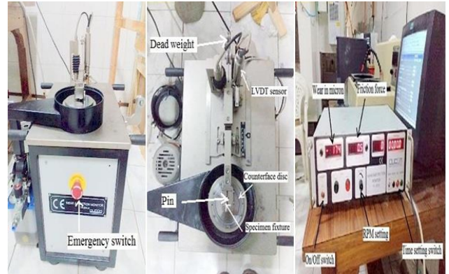
Figure 3 Components of pin-on-disk test apparatus
