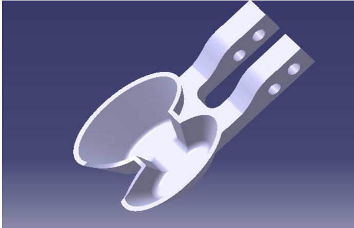
Fig 5 Pelton wheel bucket in catia work bench
