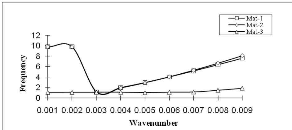
**Fig: 1** Variation of frequency with wavenumber at dissipation ( $b=0.01$ )
