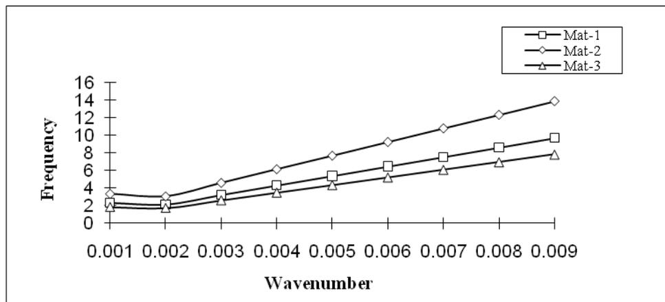
**Fig: 5** Variation of frequency with wavenumber at dissipation ( $b=0$ )
