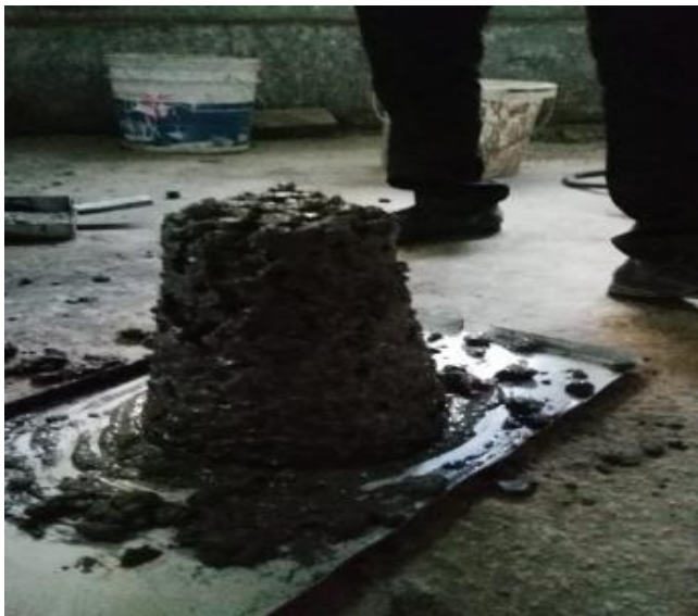
Figure 3.1 Slump Cone Test Conventional Concrete
