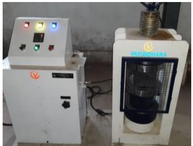
Figure 3.3 Testing Of Concrete Cubes In Compressive Strength Of Conventional Concrete Block & GGBS Concrete Blocks
