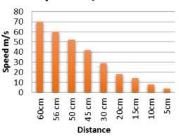
From this graph, when the obstacle is about 60cm, the speed of car remains constant. As the distance of obstacle decreases below 60cm which is detected by sensor, then the speed of car slows down. As the range of obstacle decreases below 45 cm, then the car slows down more. As this distance reaches below 15cm or below, then the speed of car decreases gradually and the motor rotates very slowly and when it comes near the obstacle, it stops near the obstacle.
