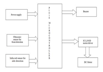
Figure 1 Block Diagram of System
