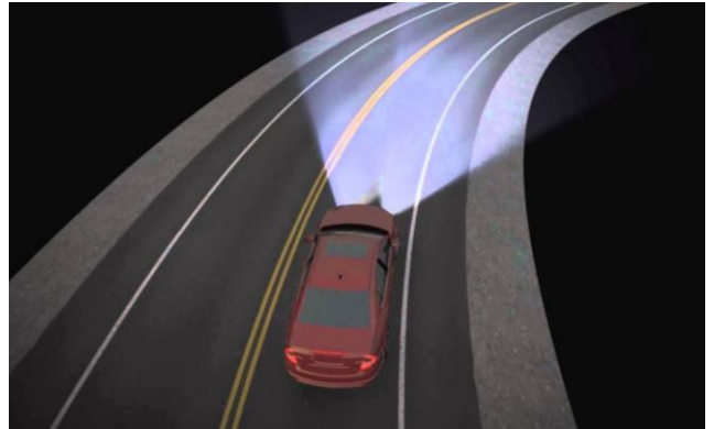
Figure 3 Adaptive Headlamp System
