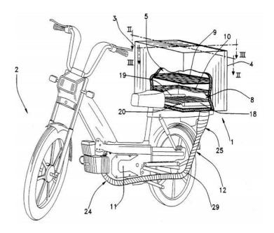
Figure 1 Food-Warming Arrangement for a Food-Delivering Motor Vehicle
