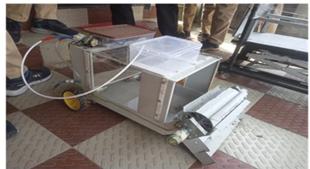
Figure 2: Automated Dung Collection 3 D design and Actual Model.
