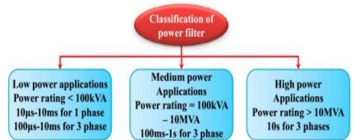
Fig. 1. Subdivision of power filter based on power rating and speed of response.
