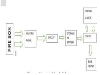
In this Block Diagram you can see when we burn waste materials and fire box then heat generating and heating panel starts to heat convert electricity and after that that electricity we can see by LED Bulb glowing and that electricity go to circuit and after that in battery and start storing power and when electricity store in battery then heating sensor turn on the output power supply and LED Bulb start glowing and smoke go to water tank and filter system start controlling pollution.
