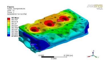
aluminium alloys). The gas side surface of cylinder wall must also be kept low to prevent deterioration of the lubrication oil film. Heat transfer effects the engine performance, efficiency & emissions. It should always be remembered that abstraction of heat from the working medium by the way of cooling the engine components is a direct thermodynamic loss.
