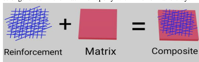
Figure 1 General formation of a composite
