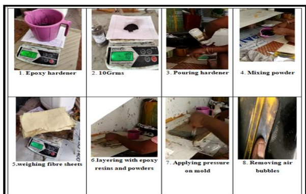
Figure 10 Complete sequential process for fabrication (1)
