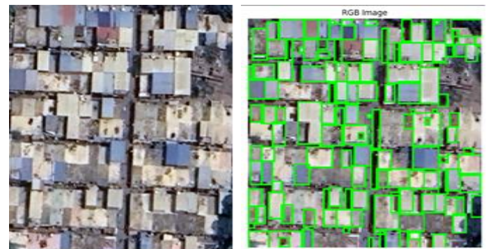
Figure 3: Rooftop Segmentation Output (SAM)
