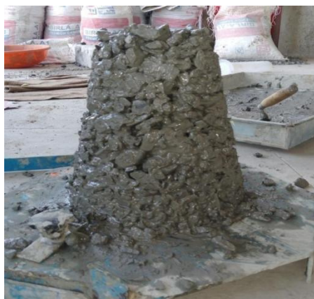
4.2.1 (b) Casting of slump cone
