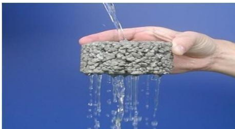
1.1.A Pervious Concrete block
