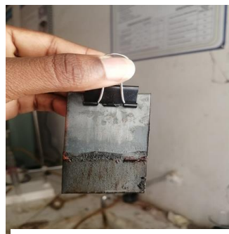
Figure 4: Coupon A state after being exposed 72 hours of immersion
