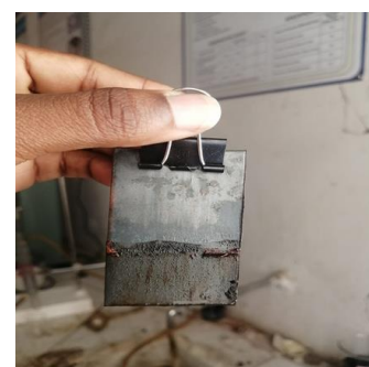
Figure 5: Coupon B state after being exposed 72 hours of immersion
