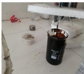
Figure 2 Coupon A being immersed in oil sample
