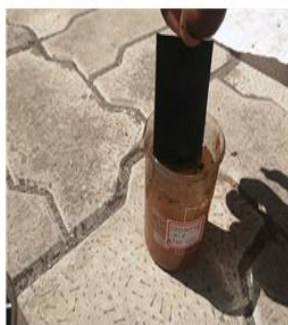
Figure 3: Coupon B being immersed in oil sample containing 2 droplets of WCI
