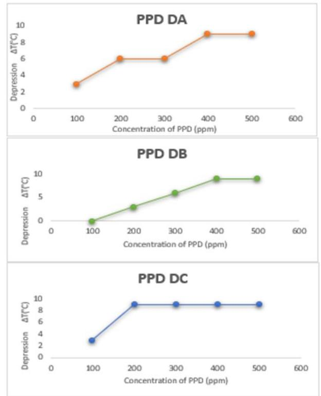
Figure 2 Graphical representation of Pour point depression  $\Delta T (^{\circ}C)$  Vs Conc. Of PPD (ppm) for DA, DB & DC
