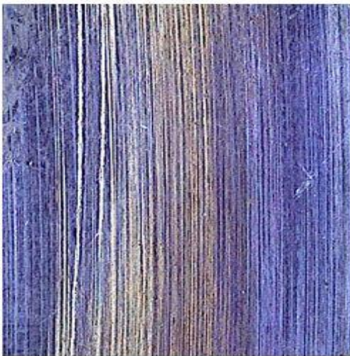
Fig. (14):-Grinding Cutting (2 Hr.30 Min. Deep Cooling)
