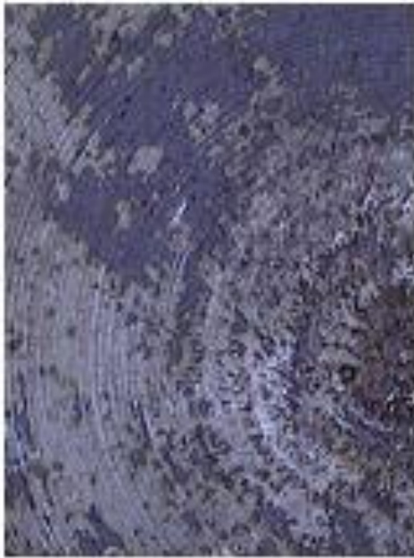
Fig.(6):- Hacksaw Cutting (30 Min. Deep Cooling)
