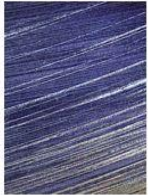
Fig.(7):- Grinding Cutting (30Min. Deep Cooling)
