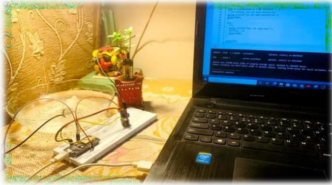
Figure 6 : Prototype of plant monitoring system using NodeMCU
