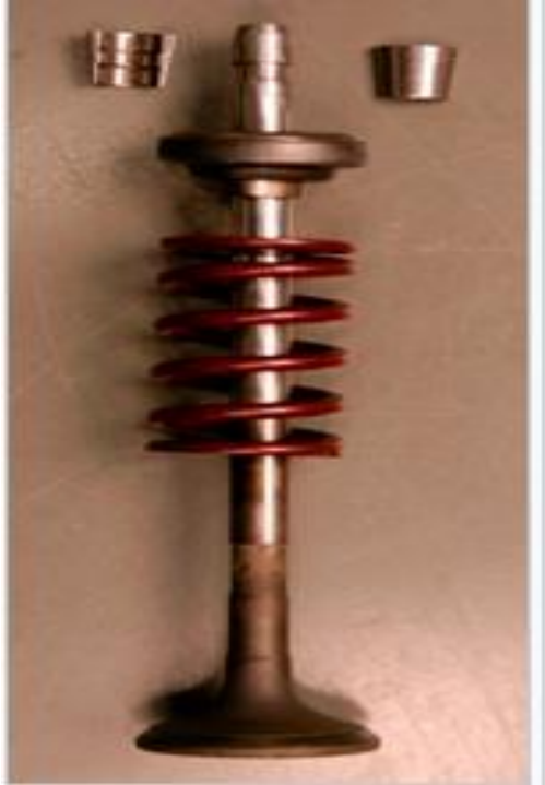
Figure 2 Poppet valve & components
