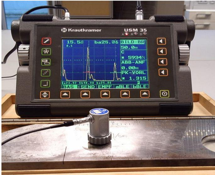
Fig.1 Experimental setup representation of USM 35X device
