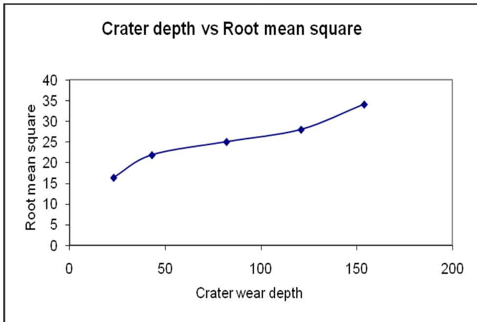
**Fig.4 Crater Depth Vs. Root Mean Square**
