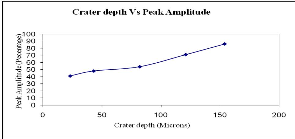
**Fig.3 Crater Depth Vs. Peak Amplitude**
