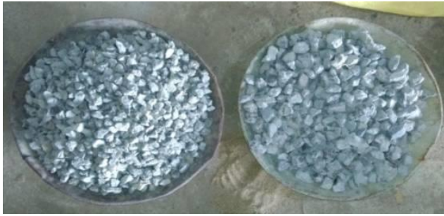
Demolished concrete aggregate
