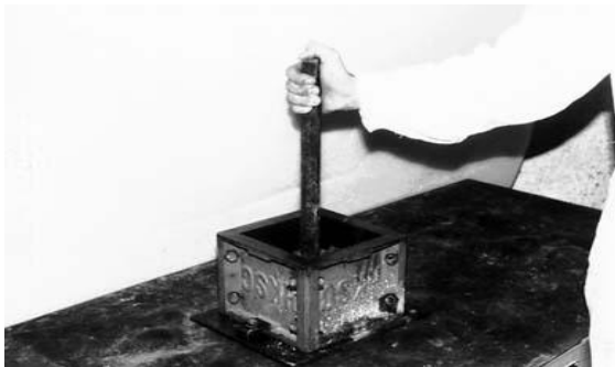
Compacting the concrete in the cube mould (For 150 mm cube at least 35 tamps per layer)
