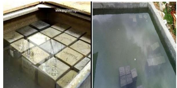
Curing of cubes and cylinders
