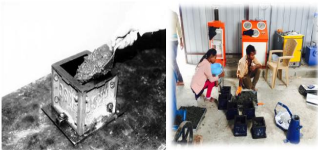
Filling the mould (for 150 mm cube 3 equal layers)
