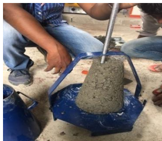
Slump cone test
