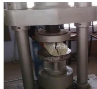
Split tensile strength of concrete
