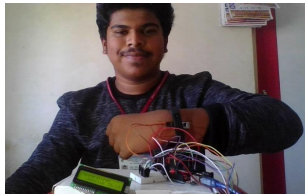
Fig. 8 Sample Band using LM35 Temperature sensor
