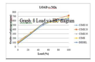
Fig 8 Load v/s NOx diagram
