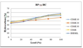
Fig 7 Load v/s HC diagram
