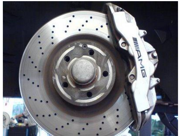
Fig 2 Disc brake with holes
