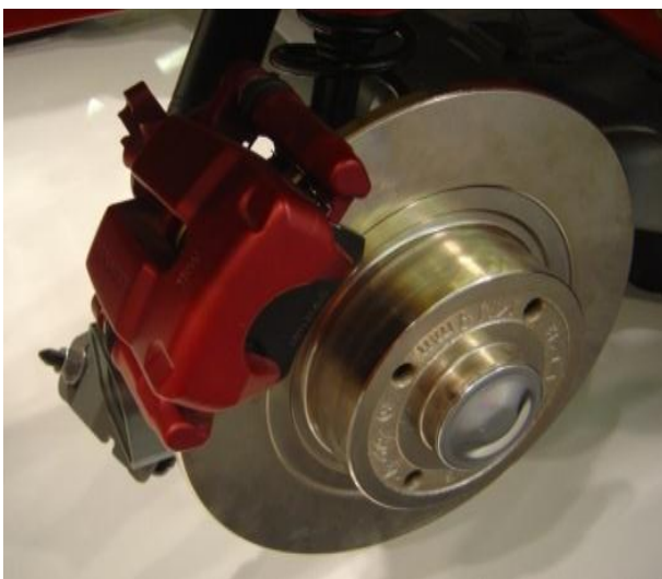
Fig 1 Disc brake without holes
