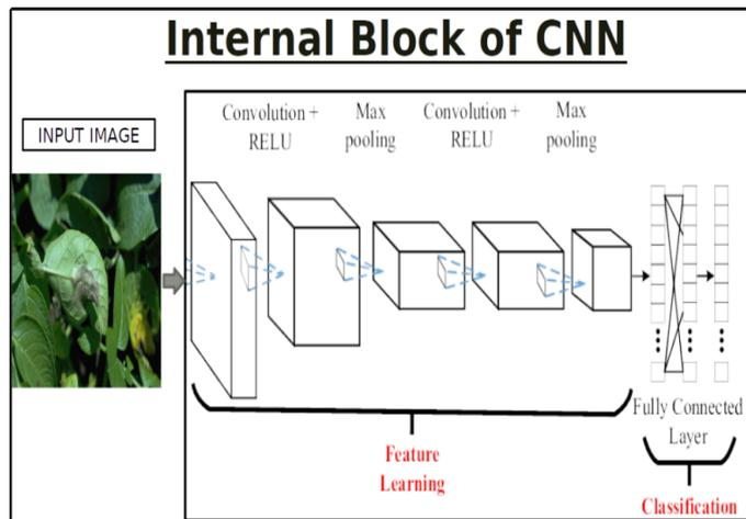
Here, we are using CNN 2D ..Basically, 2D convolutional layers take a three-dimensional input, typically an image with three color channels. They pass a filter, also called a convolution kernel, over the image, inspecting a small window of pixels at a time, for example 3×3 or 5×5 pixels in size, and moving the window until they have scanned the entire image.
