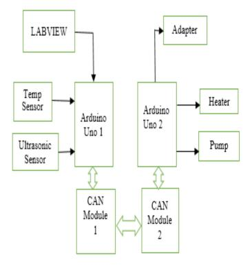
The temperature sensor LM35 and ultrasonic sensor Hc-sr04 are interfaced with Arduino Uno 1. Lm35 senses the temperature and Hc-sr04 senses the level of water in tank. After sensing data these sensors send data to Arduino Uno 1. Arduino Uno 1 transfer the data to Arduino Uno 2 through CAN module 1 and CAN module 2.
