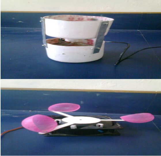
Figure 3 Wind speed Sensor and Rain gauge designed for the Project
