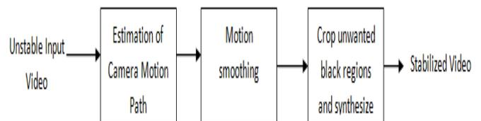
Figure 1 General Block diagram of Video Stabilization
