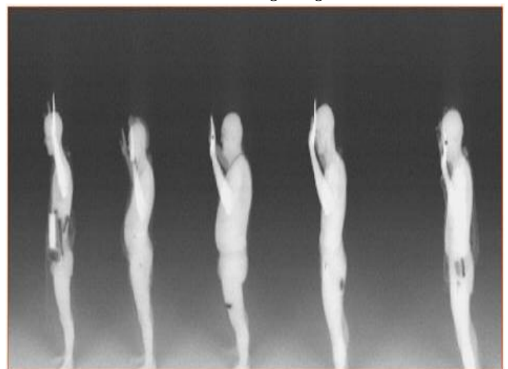
Figure 5 Standoff X-ray detection showing hidden explosives
