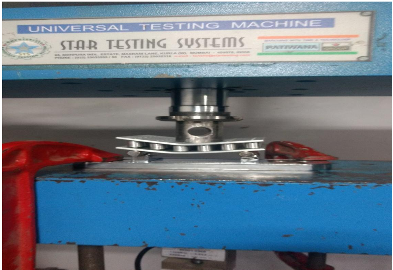
Figure.6-Bending Test on Sandwich Structure
