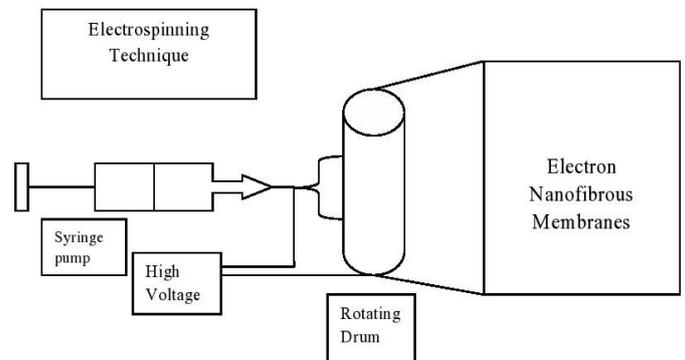
Fig. 2 Electrospinning Technique for synthesis of polymer composite
